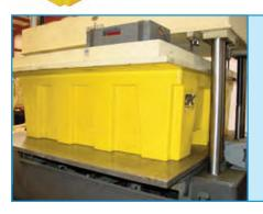
Our Spill Decks and Spill Pallets\* were compression tested to +13,500Kgs and found to be in a like new condition after testing ... or as the compression testing house said ...
